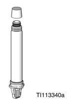
3. Insert cartridge into gun handle. Ensure cartridge tabs are aligned correctly with cartridge tab recesses in gun handle.
