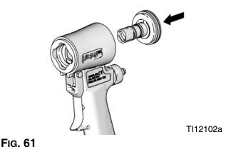
12. Install variable flow adjustment knob (X).
