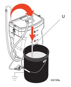
5. Lower to open the circulation handle (FC) and increase the motor air pressure regulator (MB) pressure to 20 psi (138 kPa, 1.38 bar).
