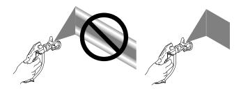
**NOTE:** Excess pressure increases overspray and pump wear.
