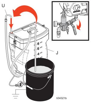
If using heaters, heat fluid throughout system before spraying. See Recirculate Prior to Spraying or Re-Prime After a Pump Runs Dry, page 34.
