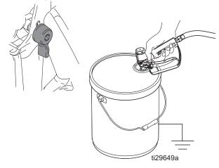
8. Close the solvent pump air valve (DA). Trigger the gun to relieve pressure. Close the solvent flush valve (FD) after relieving the pressure.
