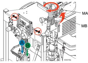
**XP-h Systems only:** Set pump valve on. Then turn down the pressure control knob.
