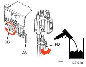
6. Open the solvent flush valve (FD)
