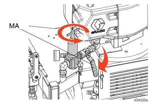
3. Make sure the solvent air valve (DA) is closed and the solvent air regulator (DB) is turned fully counterclockwise.
