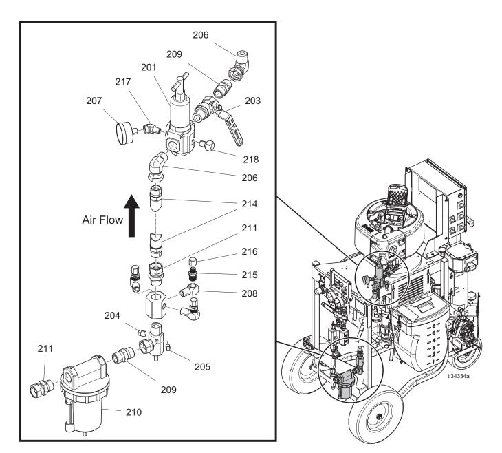
FIG. 8: Air Control Assembly 26C417
