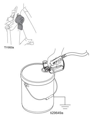
6. Engage the trigger lock. Install the tip on the gun.
