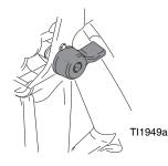
3. **XP Systems:** Turn the main pump air regulator (MB) fully counter-clockwise to shut off.
