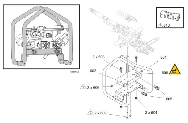
$\bigwedge$  Apply thread sealant to all non-swiveling pipe threads.
