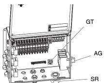
8. Verify that all items are connected properly as shown below, then close the electrical enclosure door.
