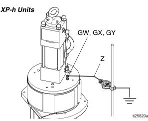
Loosen grounding lug locknut (GW) and washer (GX). Insert ground wire end (Z) into lug (GY) slot and tighten locknut securely. Connect ground clamp to a true earth ground.
