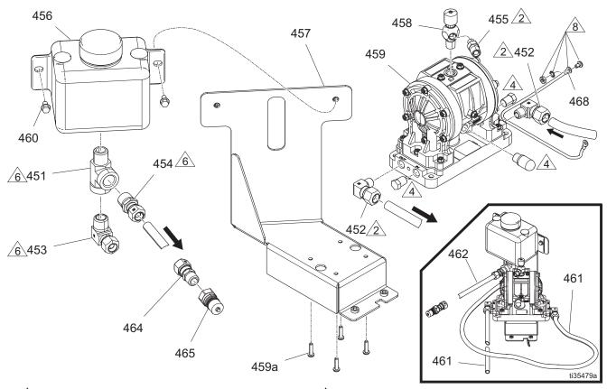
$\underline{\land}$  Apply thread sealant to all non-swiveling pipe threads.
