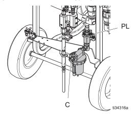
2. Remove plugs (PL) as necessary for solvent pump and feed supply pump air hoses. See pump manuals for setup instructions.
