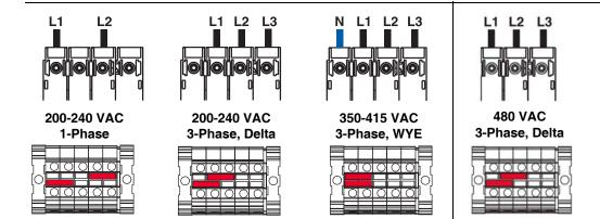
FIG. 7 Terminal Jumpers and Positions
